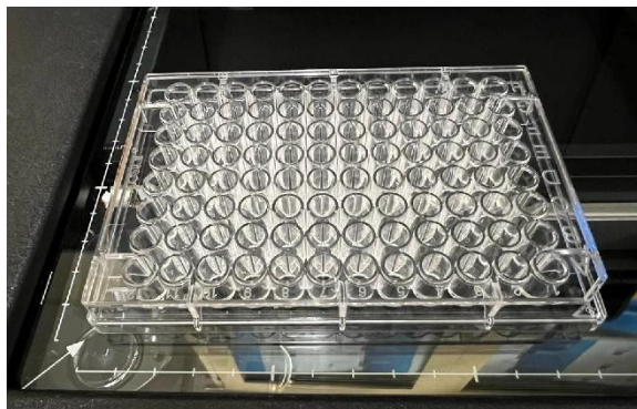
Figure 1. Plate location on LI-COR, in this case positioned in the bottom left corner.
